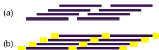
Figure 6.6: The schematic illustration of (a) pure collagen fibril and (b) mineralized collagen fibril with the hydroxyapatite platelets deposited in the gaps (Buehler, 2007).
