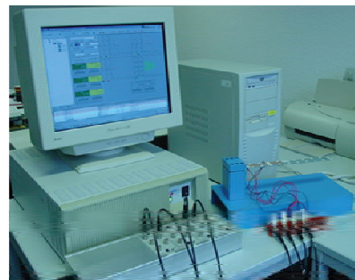
Fig. 2 Experimental rig with the clamped cantilever beam and dSPACE system
