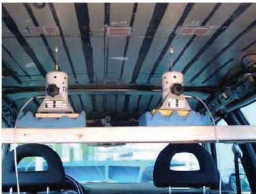
Fig. 8 Passenger compartment and inner surface of the car roof with attached piezo-patches and exciting shakers
