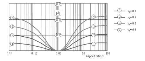
Figure 1: Accuracy of the approximate representation of the pore compliance tensor **H** as a function of pore aspect ratio  $\gamma$  for several values of  $\nu_0$
