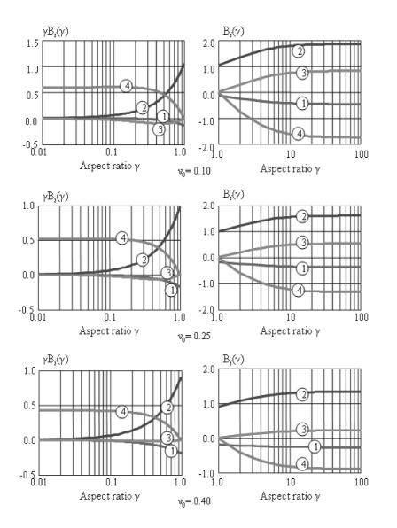
Figure 2: Factors entering approximate expression (3.1) for the compliance contribution tensor **H** as functions of pore aspect ratio  $\gamma$  and Poisson's ratio of the matrix  $\nu_0$ . Curves 1, 2, 3, and 4 correspond to  $B_1$ ,  $B_2, B_3$ , and  $B_4$ . For oblate shapes ( $\gamma < 1$ ) factors  $B_i$  enter in product with pore aspect ratio  $\gamma$ , to avoid degeneracy for small  $\gamma$
