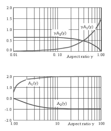
Figure 3: Factors entering expression (2.11) for the resistivity contribution tensor as functions of pore's aspect ratio  $\gamma$ . For oblate shapes ( $\gamma < 1$ ) factors  $A_i$  enter in product with pore aspect ratio  $\gamma$ , to avoid degeneracy for small  $\gamma$
