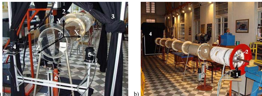
Figure 3. a) Stereo PIV configuration for calibration: 1- Nd:Yag laser power supply, 2- laser head, 3- chamber, 4- left camera, 5- right camera, 6- II-shaped camera carrier with computer controlled linear guide, 7- target and b) PIV seeding: 1- atomizer, 2- axial fan, 3- pipe, 4- measuring chamber.
