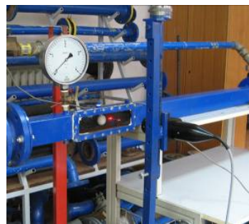
Figure 2. Measuring section of LDA test set.
