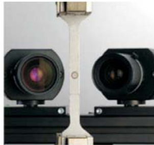
Figure 1. Video cameras "Aramis" with the tested sample at the centre [1]
