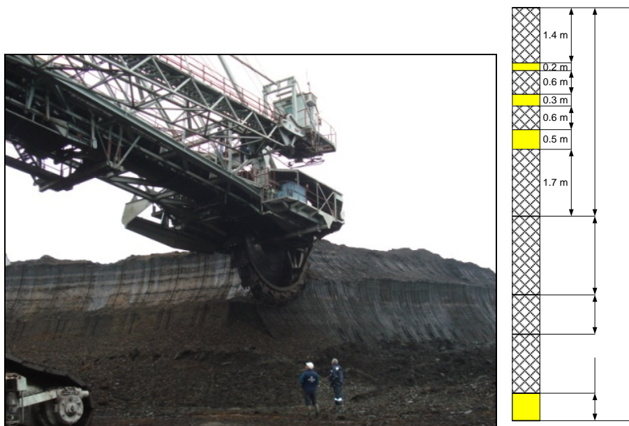
Figure 1. Vertical cross-section of the coil-block and excavator SchRs630
