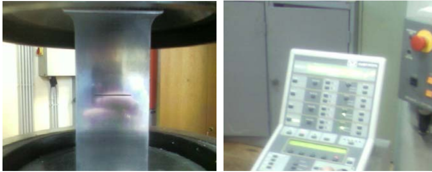
Figure 3. Tensioning specimen in testing machine with controlled growth force and stereometric monitoring crack growth.
