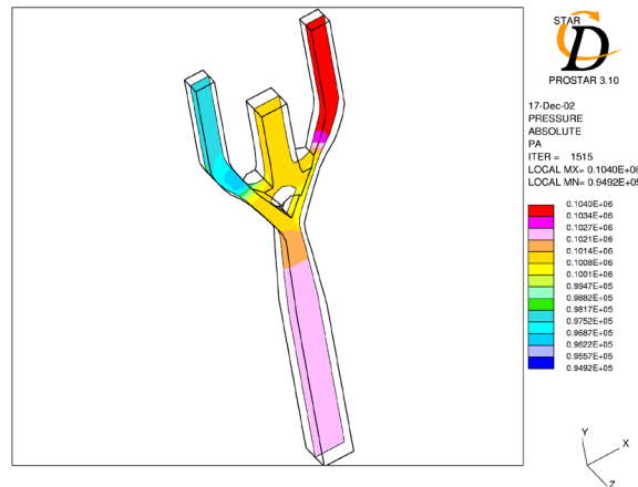
Fig. 4. Pressure field in the middle cross-section of FDV [1].
