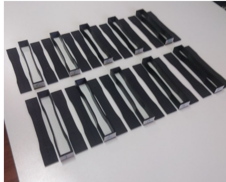
Fig 2. Moulds for production of testing specimen
